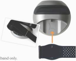
**User Tip:** Mini USB on charging dock is for use with the lark wristband only. Charge the lark wristband only with the supplied charging dock and power cord.
